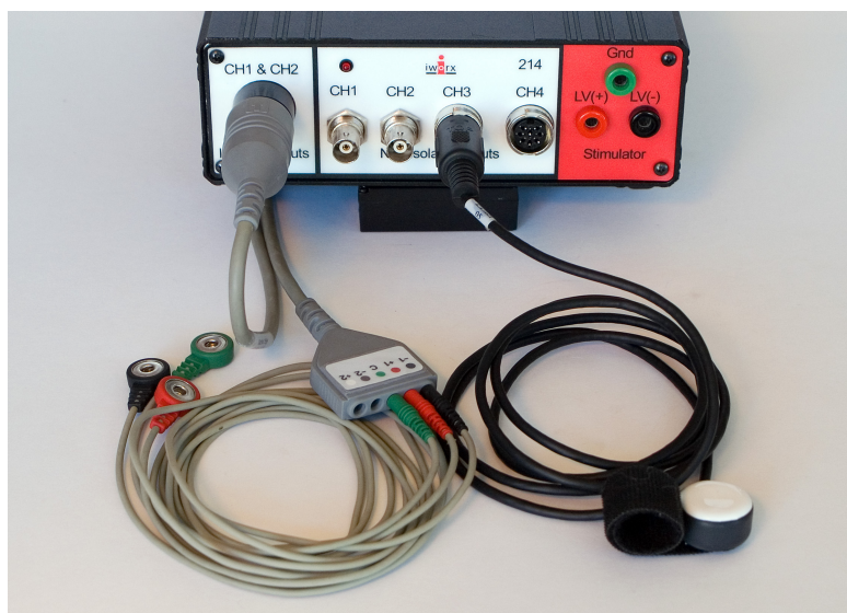
Figure HH-1-S3: The ECG cable and pulse transducer connected to an IWX/214.
